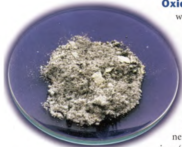
Figure 15 Calcium oxide, or lime, is produced when calcium burns in the presence of oxygen. In this reaction, the calcium is oxidized and the oxygen is reduced.
