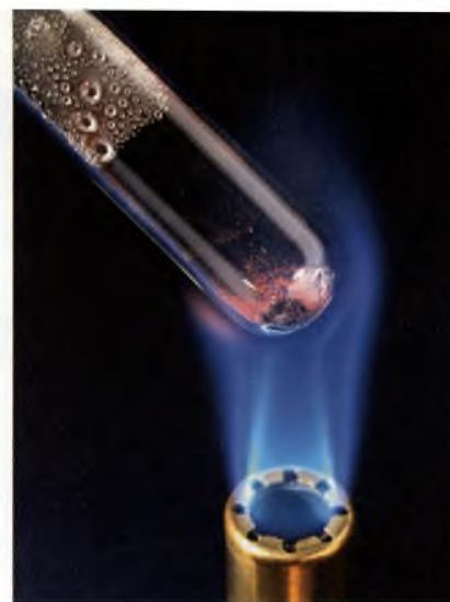
Figure 19 The orange-red powder in the bottom of the test tube is mercury(II) oxide. At about 450°C, mercury(II) oxide decomposes into oxygen gas (which escapes from the test tube) and mercury (droplets of which can be seen collecting on the sides of the test tube).
