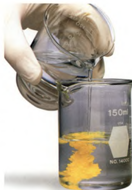
Figure 13 When potassium iodide solution is poured into a solution of lead(II) nitrate, a double-replacement reaction takes place. Lead(II) iodide forms as a yellow precipitate.
