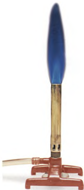
Figure 14 A Bunsen burner generates heat and light by the combustion of natural gas.
