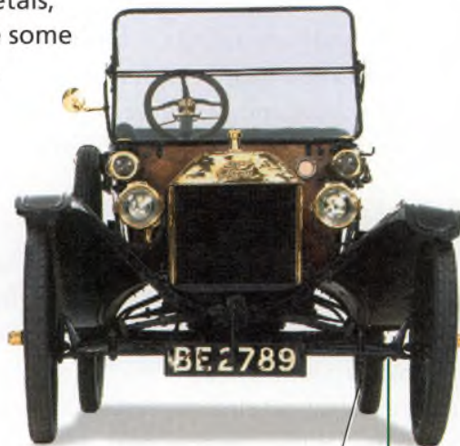
Vanadium steel This alloy becomes popular in car manufacturing because it is lightweight and strong.
