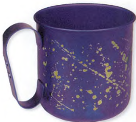
Figure 1 The handle and body of this titanium mug were welded together in an argon atmosphere. If titanium is allowed to react with oxygen in air, the compound that forms makes the weld more brittle and more likely to break.
